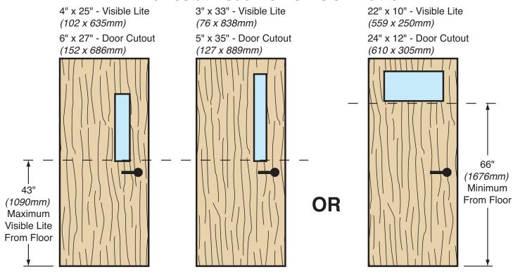
The above drawings are based on 3-0 x 7-0 doors, and are drawn to scale.
