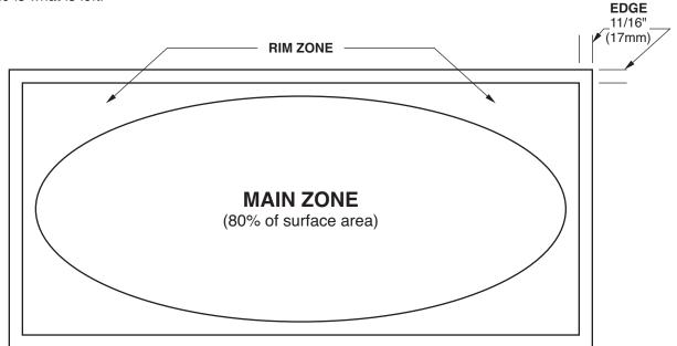
When inspecting a piece of glass you should be standing 10 feet (3.1m) from the surface of the glass and at a 90 degree angle perpendicular to the glass surface. (Inspection Guidelines Similar to ASTM Standard C 1376)
