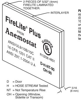
PLEASE NOTE: On visible lite sizes larger than 1296 sq. in. (0.836 m<sup>2</sup>) on 20/45 min. and sq. in. (0.065 m<sup>2</sup>) on 60/90/180 min., please consult with your Door / Frame Manufacturer's procedures, for their maximum glass size tested.
