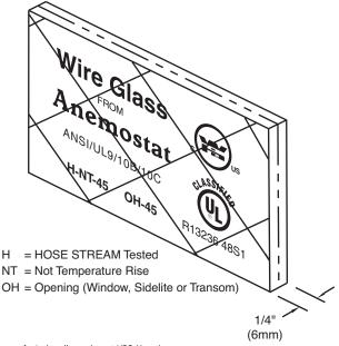
Anemostat manufacturing dimensions ±1/32 (1mm) Actual dimensions are nominal and may vary based on component manufacturers tolerances.
