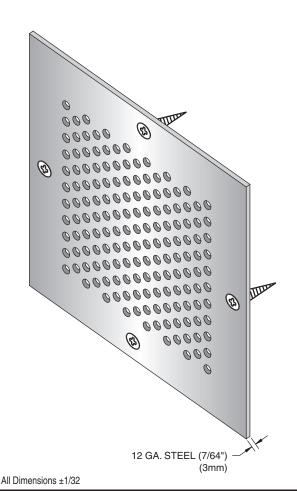
FRAME O.D. ORDER SIZE WIDTH OPENING AREA ORDER SIZE LESS 2 3/8" (60mm) 00000000000000 ORDER SIZE LESS 2 3/8 00000000000000 0000000000000 00000000000000 00000000000000 **FRAME** O.D. LESS 2 3/8 **ORDER** SIZE 3/8" **HEIGHT** (10mm) 0000000000000 (60mm) 000000000000000 0000000000000 00000000000000 0000000000000 00000,0000000 1 3/16" (30mm) 5/16" (8mm) DIAM. HOLES ON 7/16" (11mm) STG. CTRS. 1 3/16" (30mm)
